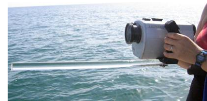
Figure 1. A Plexiglas rod helps the videographer maintain a fixed distance of 40 cm off the bottom.
