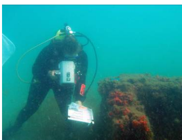
Figure 2. The videographer films a slate that identifies each site and transect prior to capturing the footage used for the analysis.
